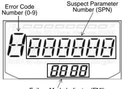
If the CHECK ENGINE light illuminates, retrieve the error codes from the display.
